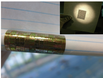
Fig. 1: Array of 12 CMOS chips transferred onto a paper sheet using the UTTBT method. Excellent bendability is demonstrated by winding the host paper substrate on itself. (Insert) Transparency is obtained over the chip area not fully covered by the metal interconnection layers.
